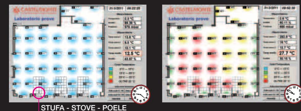
The pictures show our laboratory tests that verify the uniform distribution of heat in a room of 95 square meters. The thermal acceleration is very fast so the average temperature of the room rose from 12.5 ° C to 27.7 ° C, in just 30 minutes.
